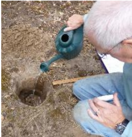
Figure C-1. Anyone fit enough to dig can perform an infiltration test with commonplace tools.
